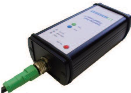
In case of AS-interface devices or 24Vdc binary devices the copying tool for motor starters and frequency inverter stored the device parameters (eg. from a master device) by a download. These cached device parameters can be uploaded to further devices which have been changed or which have been installed in a new application without a laptop or PC software. Just with a two-button function.
